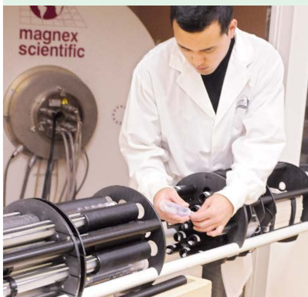
The Mouse Imaging Centre (MICE) adapts magnetic resonance and other imaging technologies for imaging of mouse models. The equipment in this photo allows scientists to image multiple mice in the same scan, greatly increasing the efficiency of their research. (Photo: CP Images/S. Lake)
