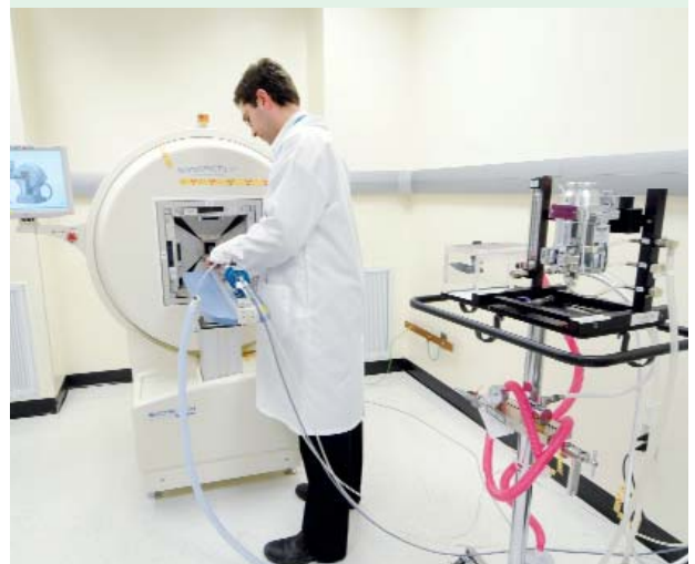
Small-animal NanoSPECT/CT scanner at the STARR facility in Toronto's Discovery District. (Photo: CP Images/S. Lake)
